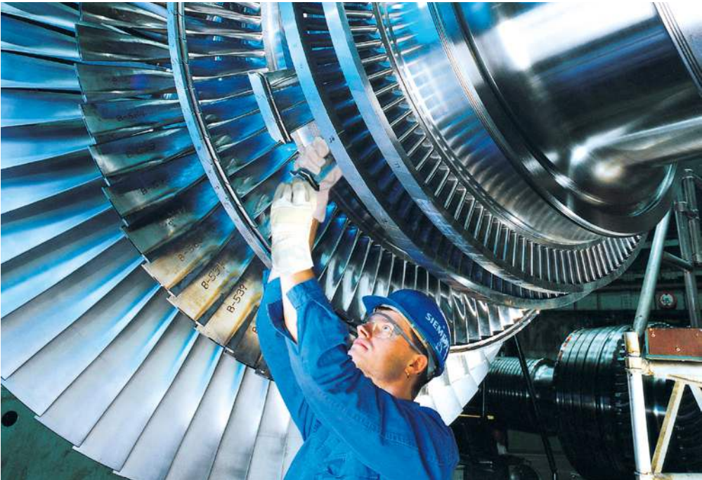
Turbine blades on a steam turbine rotor used in a power station
