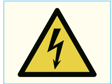
Figure 1: Warning of dangerous voltage
