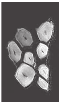
5: Flax fibres, cross-section
