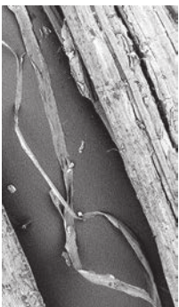
4: Flax fibres, longitudinal view
